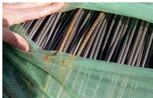
Goods after transport without VCI protection
