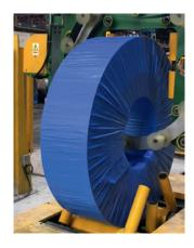
The machine provides an Automatic solution for the wrapping of Slit Coils within downstream manufacturing and service centres providing a cost-effective alternative to manual packing. Its unique and patented self-sealing system provides a strong robust anti corrosive packaging using a single packaging medium application.
