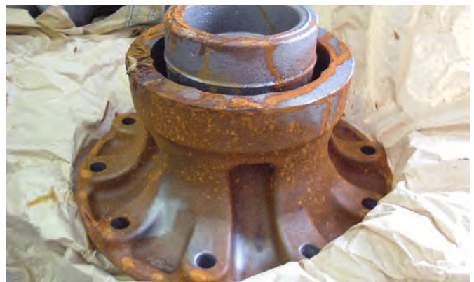
Goods after transport without VCI protection
