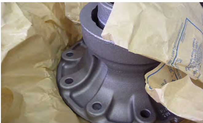
Goods after transport with VCI protection
